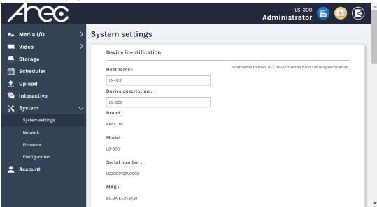
2. Check the 10<sup>th</sup> digit of the S/N. If it is "V", then the device has the new hardware. If it is "0", it has the original hardware and is not compatible with the firmware series described in this release note.
